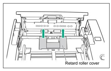
A Remove the retard roller module in the direction of the arrow.
