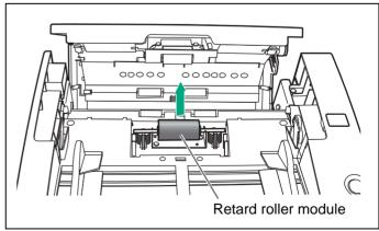
Install the new retard roller module by matching the groove of its shaft with the groove of the metal holder.
