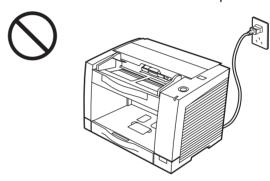
Do not place the unit on an uneven or unstable surface.
