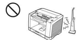
Do not place the unit on a carpet. (Static electricity can cause the unit to malfunction.)
